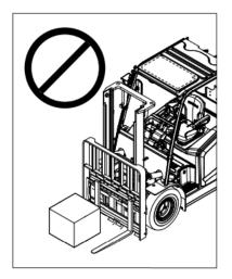
2) Do not elevate the load with the ends of the forks.
